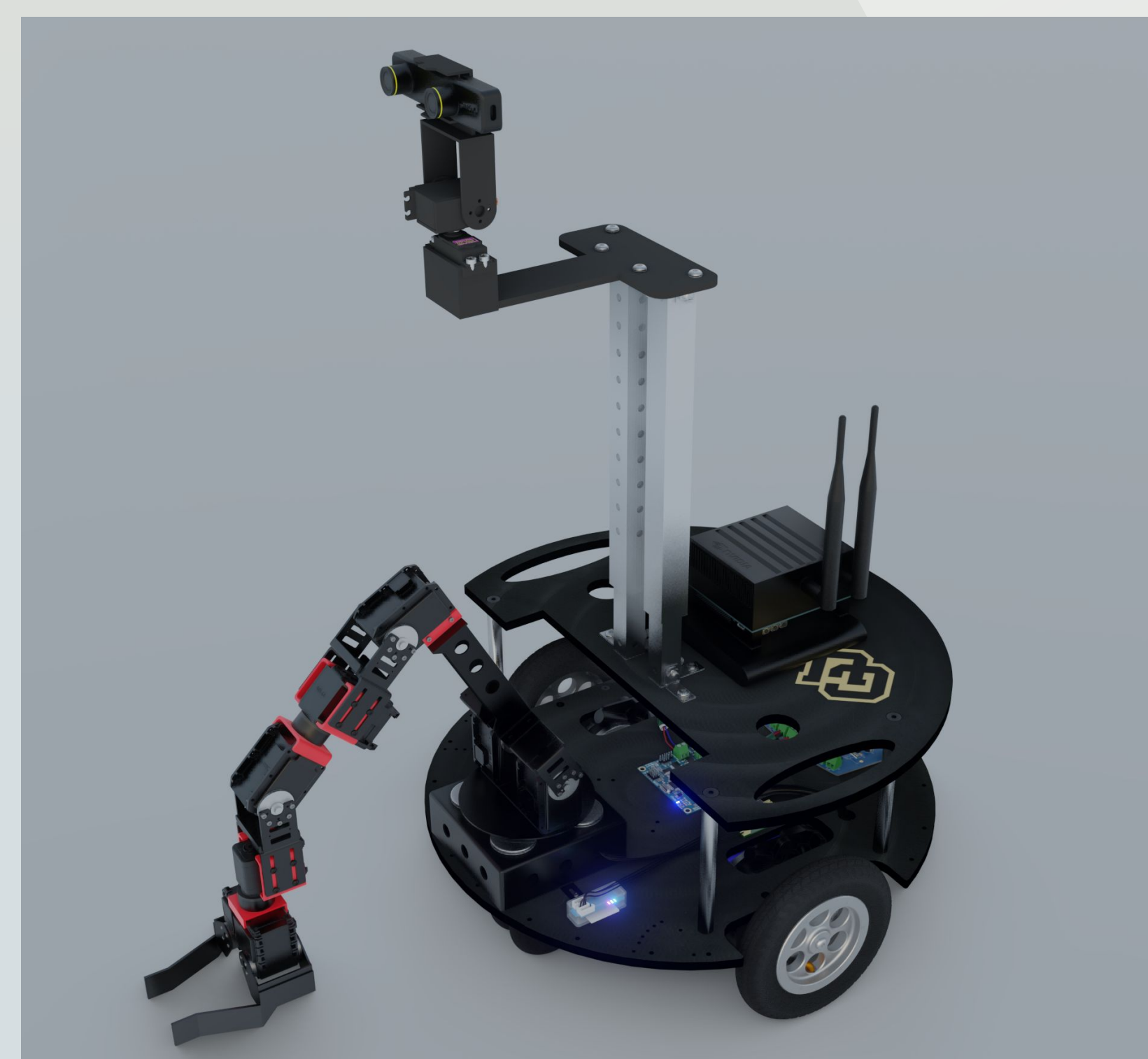
Rendered image of the Armstrong rover. This model is physically accurate for use in the virtual recovery sandbox
