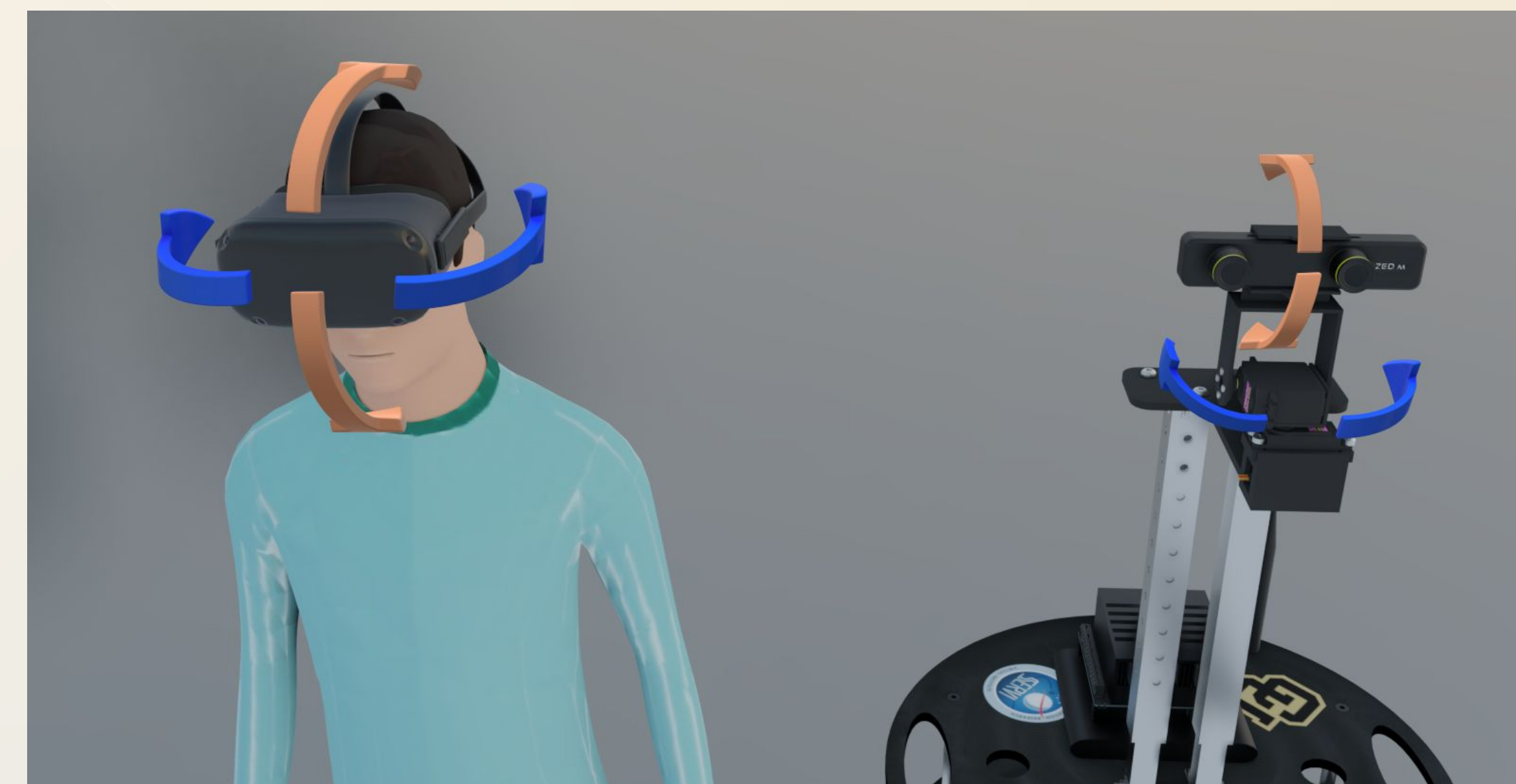
Armstrong's telepresence interface. Two servo motors help to mimic the teleoperator's viewpoint by tracking the HMD's orientation
